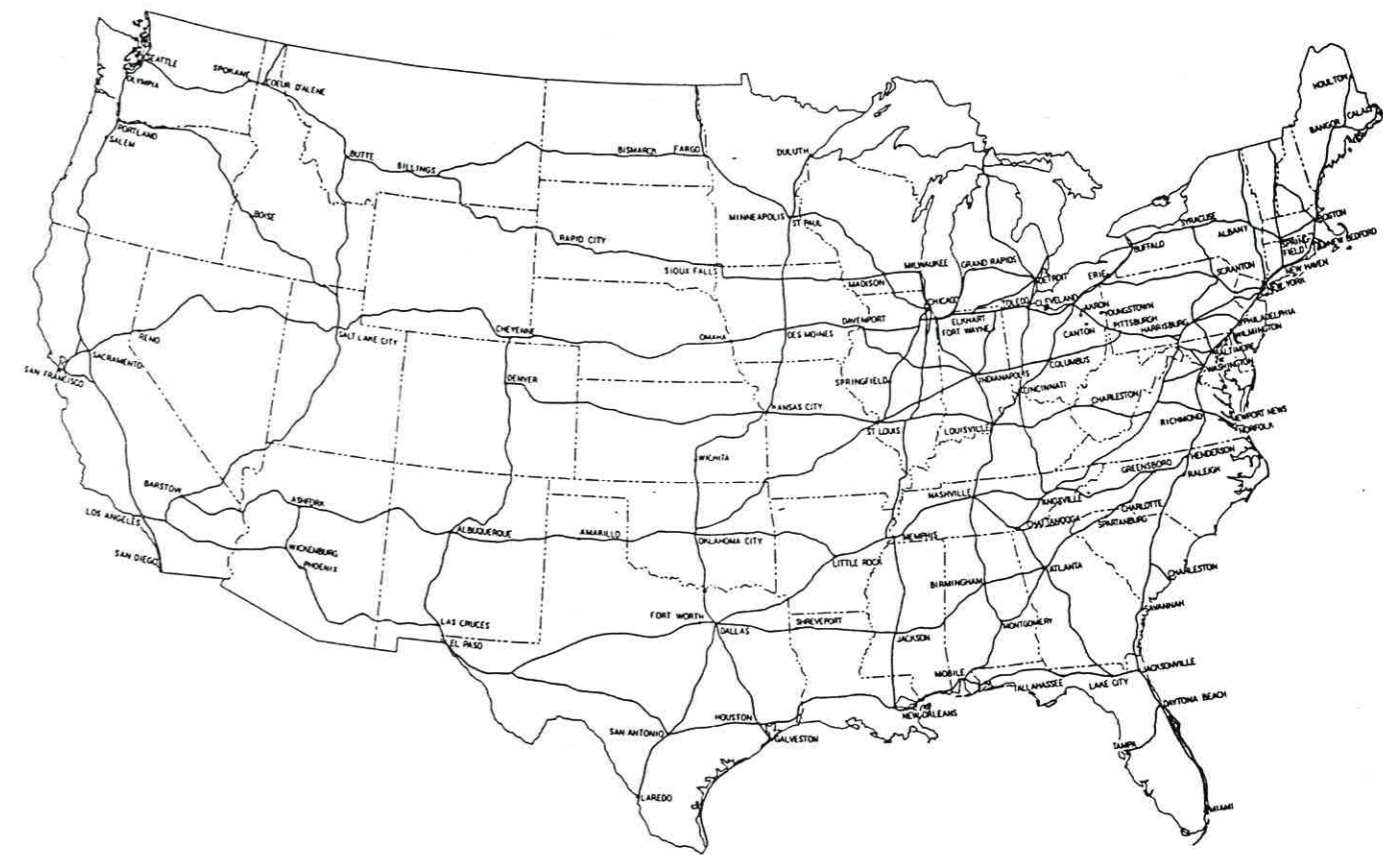
図 4-1-4 The general location of routes of the recommended interregional highway system. Total length of the system is 33,920 miles.
